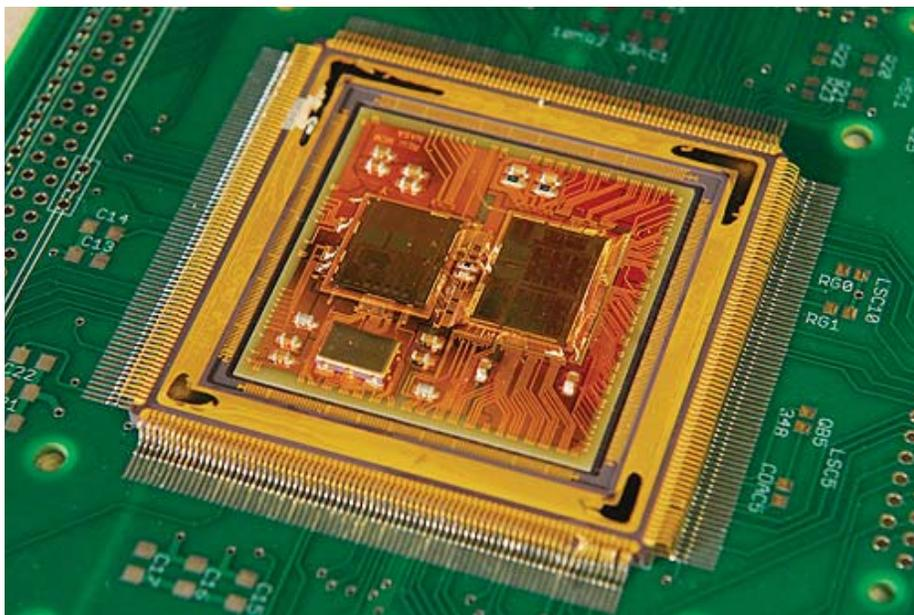
**Image 3:** This close-up image shows a remote electronics unit 16-channel sensor interface, developed for NASA using silicon-germanium microchips by an 11-member team led by Georgia Tech. (Photo: Gary Meek)
